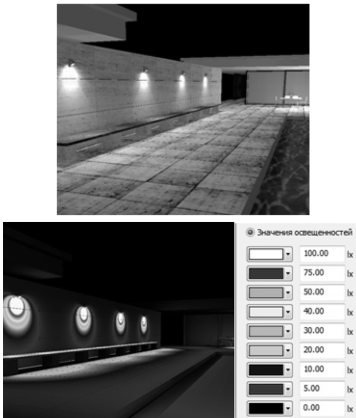
Fig. 5. 3D visualization of functional illumination and Illumination distribution levels in fictitious colors
